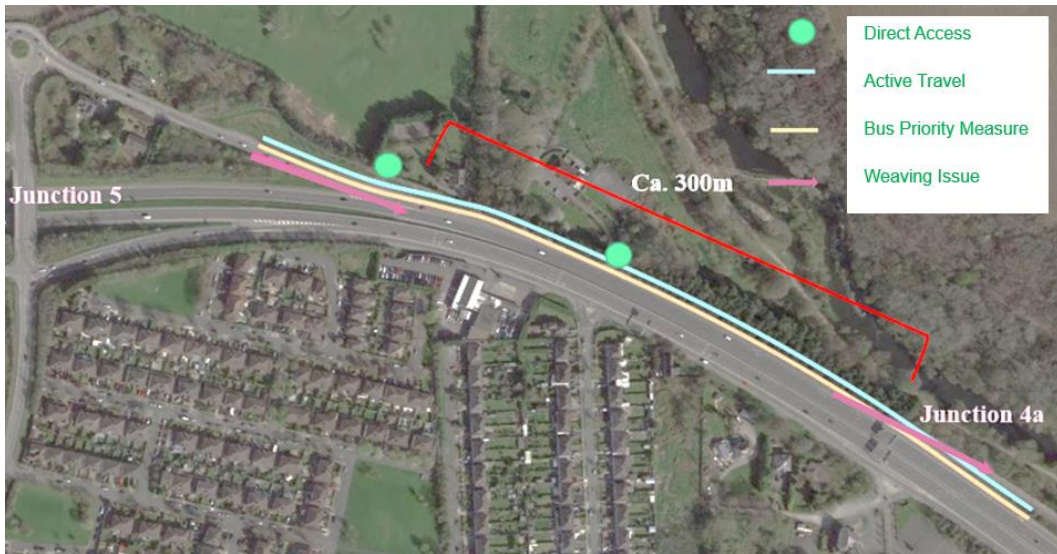
Figure 6.26: M4/N4 Junction 5 to Junction 4a Existing Layout
