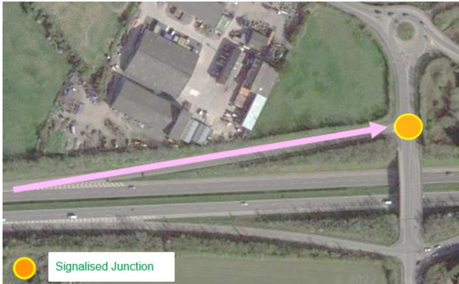
Figure 6.18: Eastbound Diverge Scenario 1 - Amend from 1 Lane Diverge to 2 Lane Diverge and Signalise Junction
