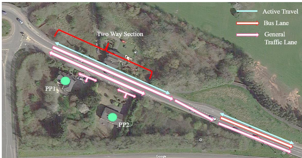
Figure 6.17: Eastbound Merge Existing Layout
