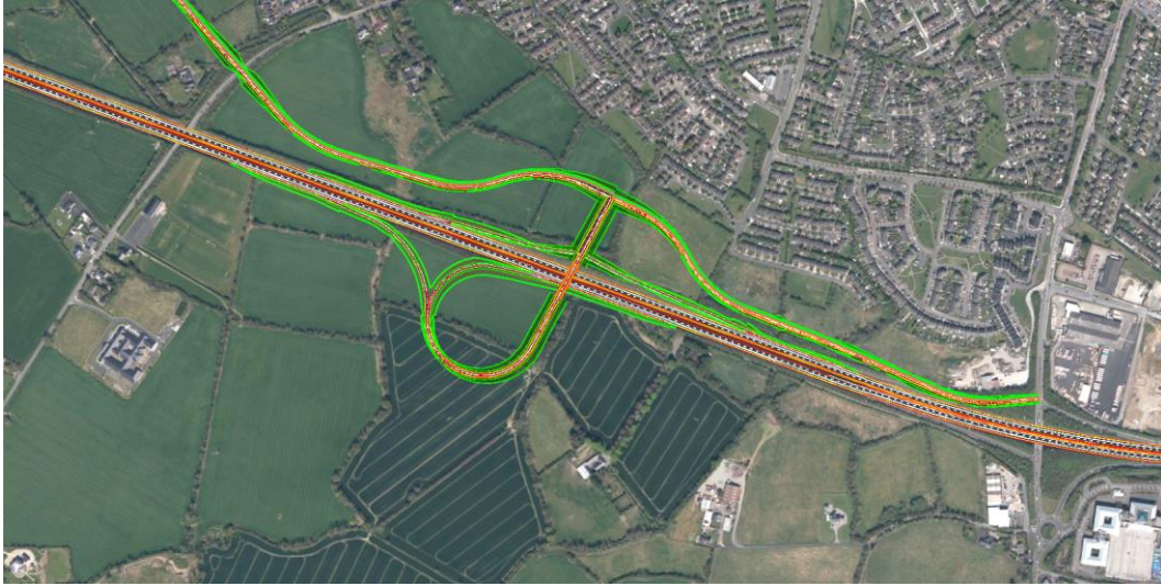
Figure 6.9: Option 2 - Linkage to the North - Signalised Diamond on northern side and Loop on southern side (© Google Imagery ©2024 DigitalGlobe)
