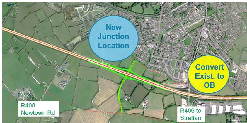
Figure 5.37: Option 2 - Provide 1 New Junction and Convert Existing to an Overbridge (1 Junction Option)
