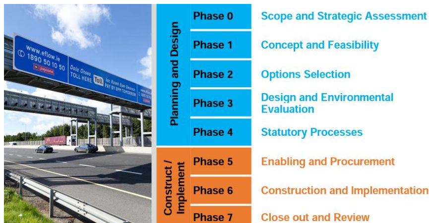
Figure 1: TII PMG Project Phases
