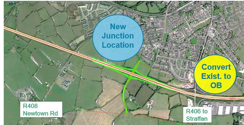
Figure 5.18: Option 2 - Provide 1 New Junction and Convert Existing to an Overbridge (1 Junction Option)
