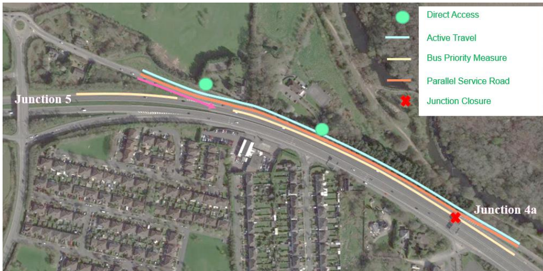
Figure 6.27: M4/N4 Junction 5 to Junction 4a Parallel Service Road
